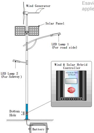
Esavior 400W wind turbine mainly applied in wind/solar hybrid street light.
